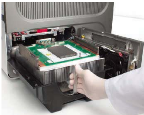
▲ LightCycler® 480 Thermoblock for 96 or 384 wells, easily exchanged by users within minutes.
